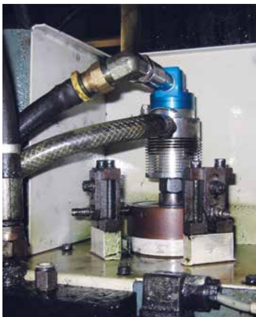
DEUBLIN 1109 on vertical machining center
