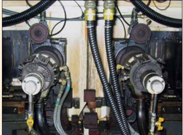
DEUBLIN 2-passage Unions on CNC Turning Center
