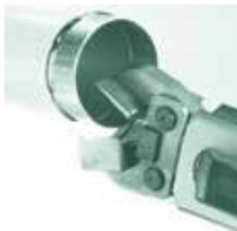
Manually open the jaw and insert the stainless steel pipe until the pipe meets the stop in the jaw.
