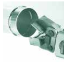
Re-open the jaw to remove the pipe. Position the end of the jaw next to the lug mark: this will help to prevent overlapping the lugs.
