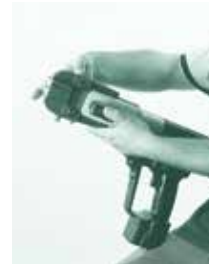
Lock into position by closing the retaining pin.
