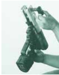
Open the retaining pin at the front of the machine by pressing the jaw to release button*.
