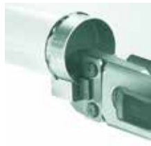
Release the jaw then press the trigger and lug the pipe until a "snap" is heard.
