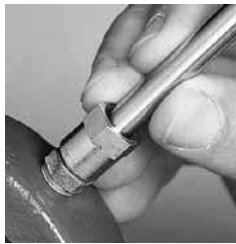
3. Seal and tighten Zerk-Lock using a hammer and staking tool
