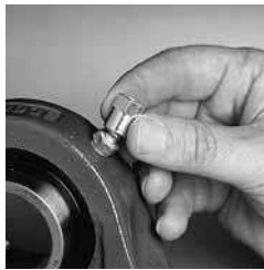
2. Place a Zerk-Lock onto the fitting
