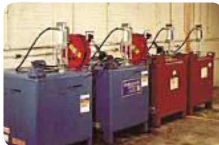
Transferring fluid lubricants and grease from bulk tanks is both cost effective and environmentally sound. These bulk tank systems help to eliminate drum disposal and the meters will track the volume of lubricant that is dispensed for each product.
