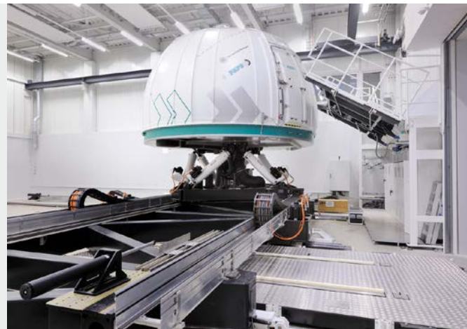
ACE safety shock absorbers protect end positions in two axes of a driving simulator Bosch Rexroth BV, Boxtel 5281 RV, The Netherlands and University of Stuttgart - FKFS, 70569 Stuttgart, Germany
