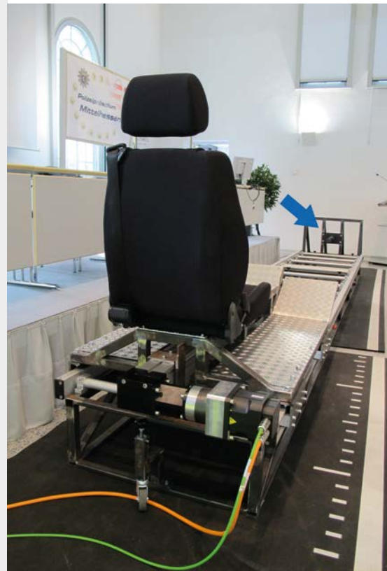
MAGNUM dampers ensure the reliable braking of moving masses on the seat and the protection of the entire carriage construction Central Hessian Police Department, Karl-Glückner-Straße 2, 35394 Gießen, Germany
