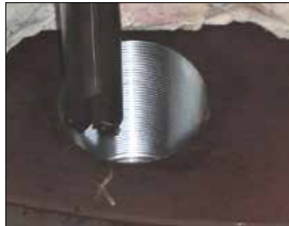
▲ New machined thread
