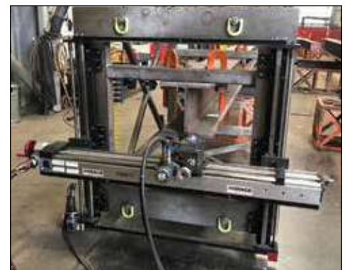
I-Beam end face milling with a GMRF1000. ▶
