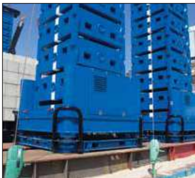
▼ Enerpac JS500 used in bridge construction and de-commissioning.
