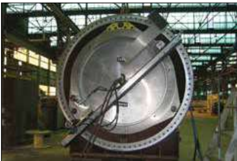
▼ Wind tower machining with WP4600.
