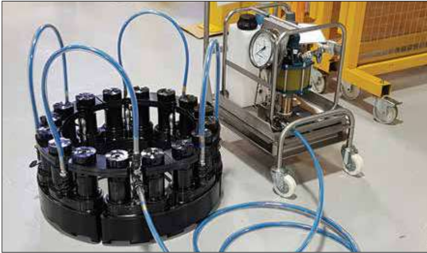
▲ Multi Stud Tensioning Set-Up.
