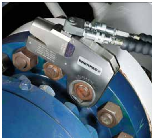
◀ The ZE4 torque wrench pumps are perfectly matched for this W2000X wrench.
