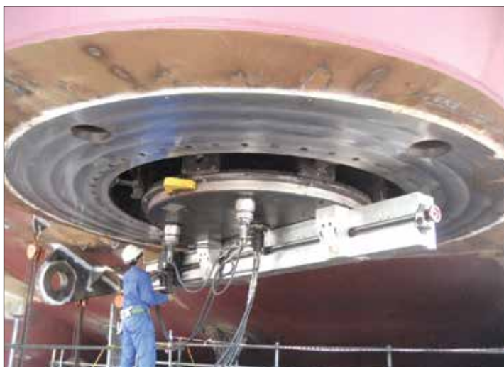
▼ Milling a ship thruster flange.
