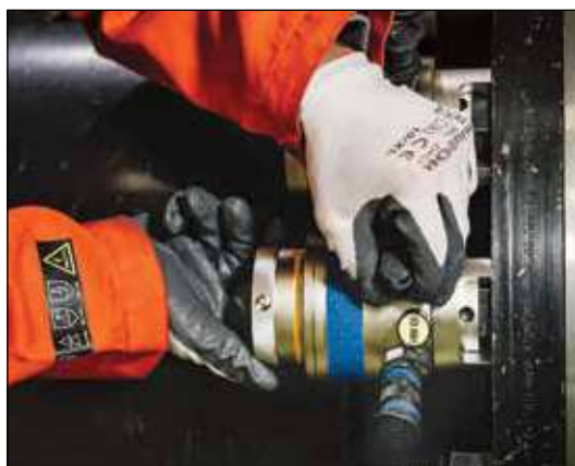
◀ Enerpac HM-Series HydraMax® tensioners have been designed to generate high-bolt loads associated with compact flanges, while providing versatility for maximum bolt coverage.
