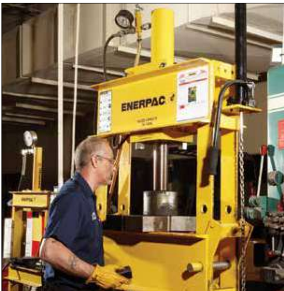
◀ An Enerpac H-Frame press quickly removes the shaft from this assembly.
