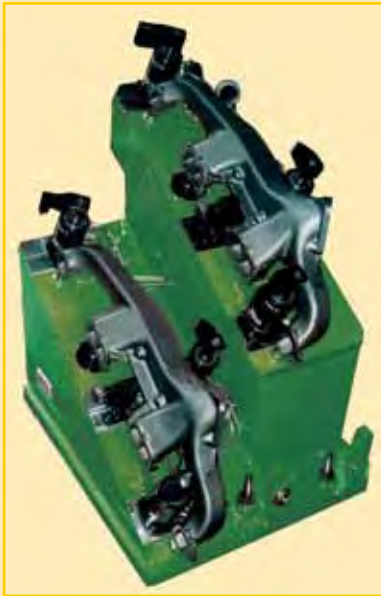
■ Fixture for machining exhaust manifolds.
