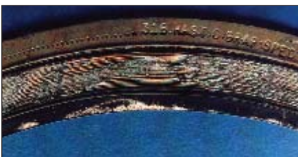
Oxidized spiral wound gasket
