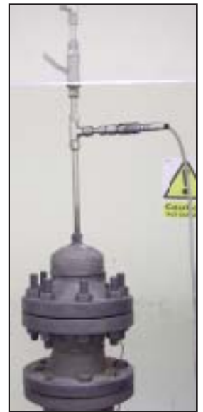
Thermal Cycle Rig • 4” Class 300 • B16 Studs • Internal heating element
