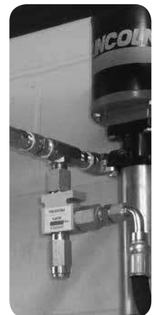
Thermal relief kit shown on PMV pump
