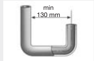
● Minimum clearance of U-shape bends
