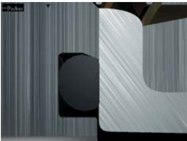
After tightening the nut Standard O-Rings can be fitted instead of "Trap Seals"
