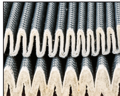
Photo above shows 'dry' Par-Gel filter media and the same media swollen with absorbed water.
